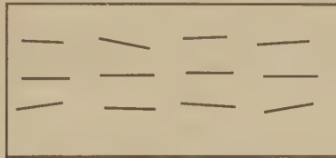
Paramagnetic substance becomes even more aligned in the magnetic field of a CGS meter.
