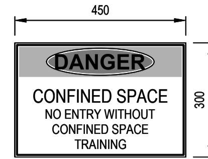
CONFINED SPACE SIGN SCALE 1: 10
