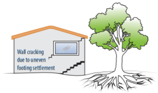
FIGURE 1 Trees can cause shrinkage and damage.
