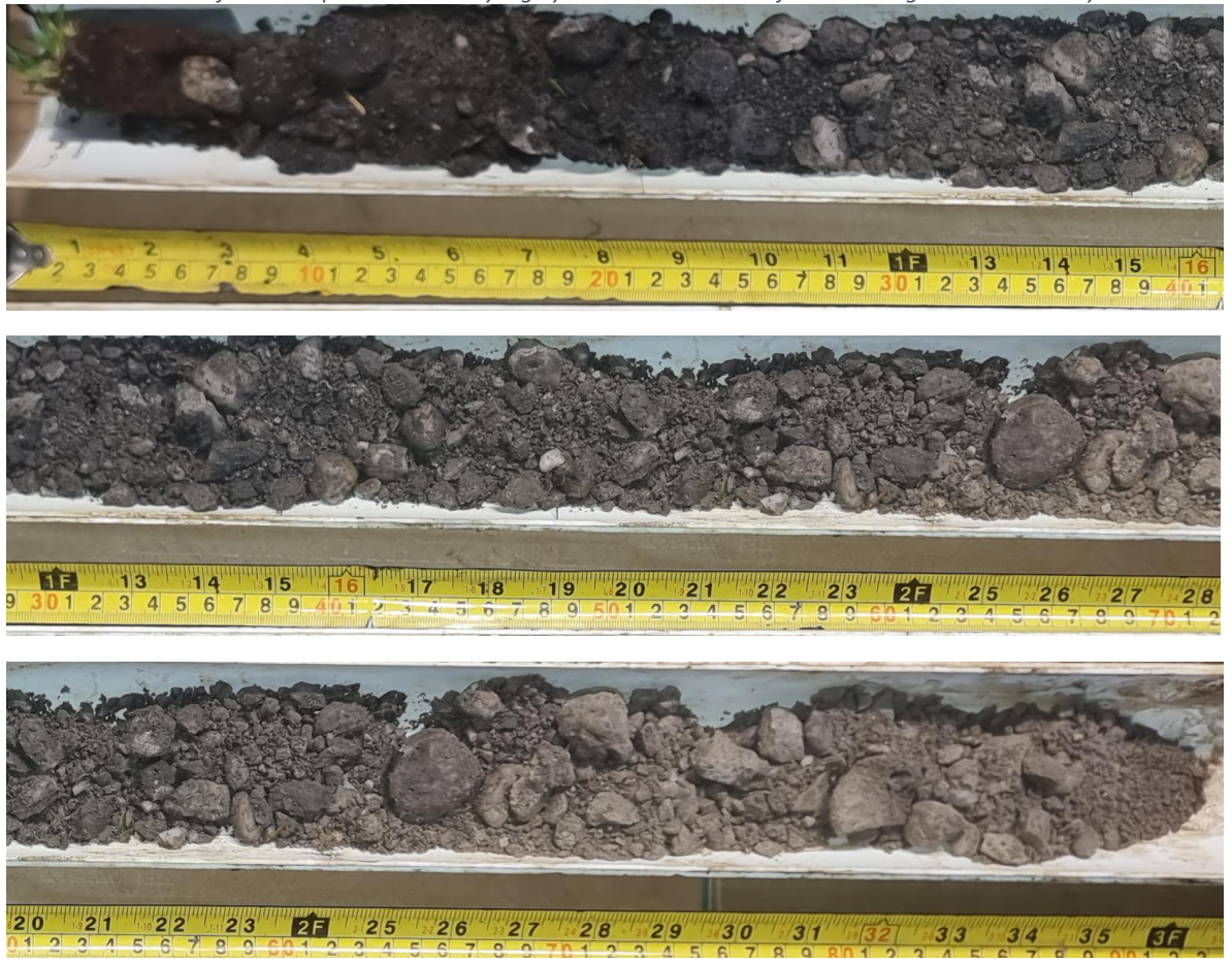
Figure 5. TH2 lithology transitions at 0.1m, 0.3m, & 0.6m with refusal at 0.95m. Stabilised aeolian coastal sand atop marine sands. Base of core sample dominated by highly weathered rock that features a slight increase in clay alteration.
