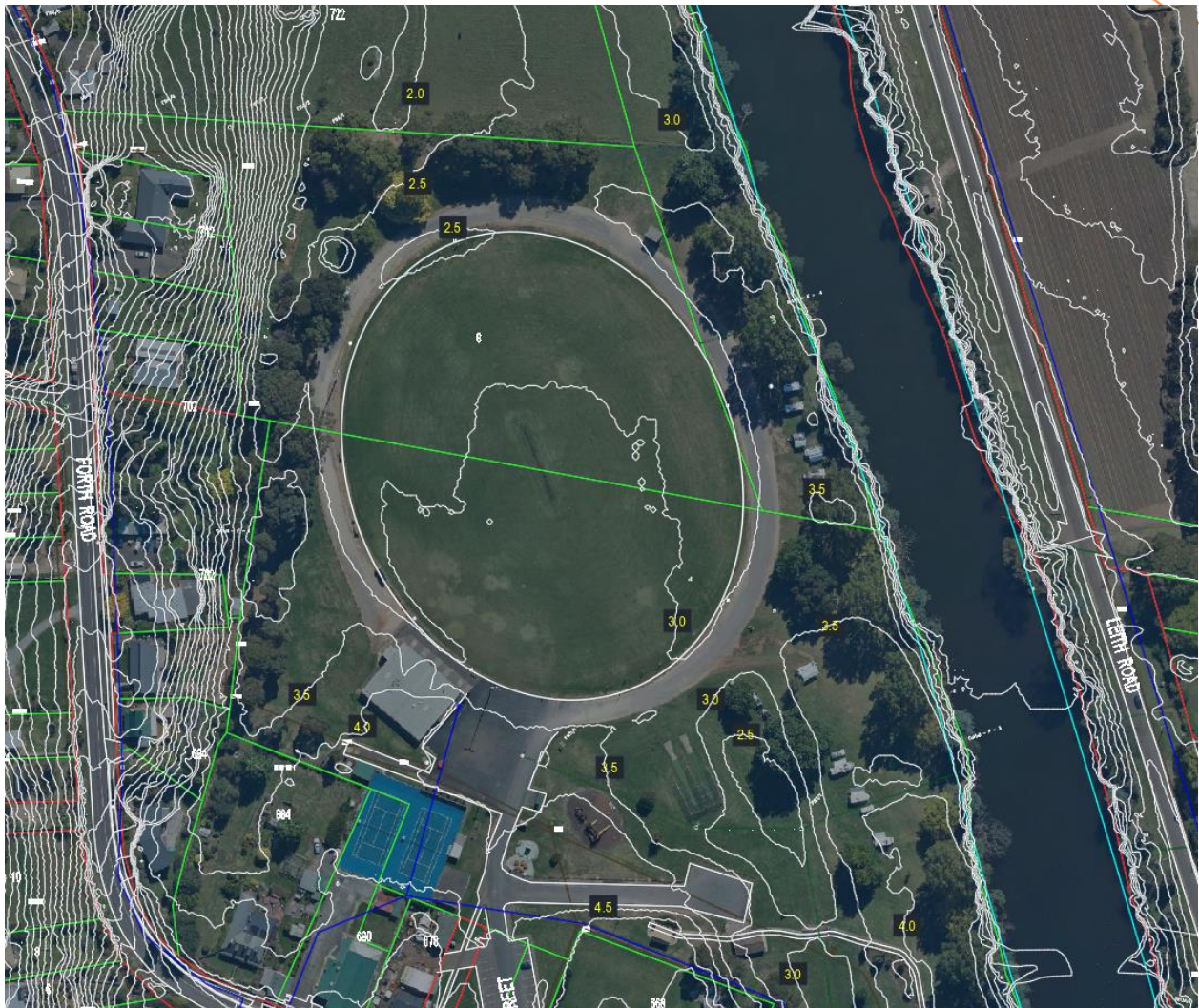
Figure 5: Aerial photo of Forth Oval showing the existing site levels (Adapted from the original, sources – Geoscience Australia, 2022 and 'GoogleEarth Pro', 2022)
