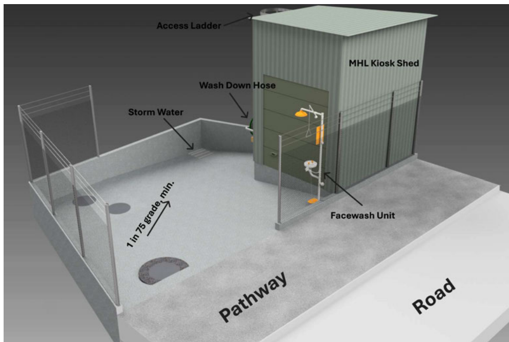
Figure 4 – MHL Kiosk General Arrangement
