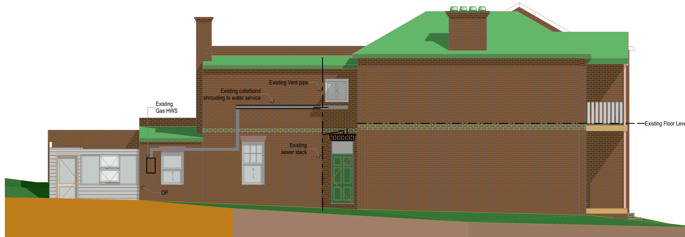
Existing South Elevation
