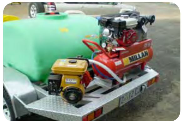
Mobile washdown units with high pressure pump, hose and compressed air unit (for blow down of slasher decks, interior, air cleaners, radiator grills etc). Photo courtesy of NRM South/Southern Tasmanian Councils Authority.
