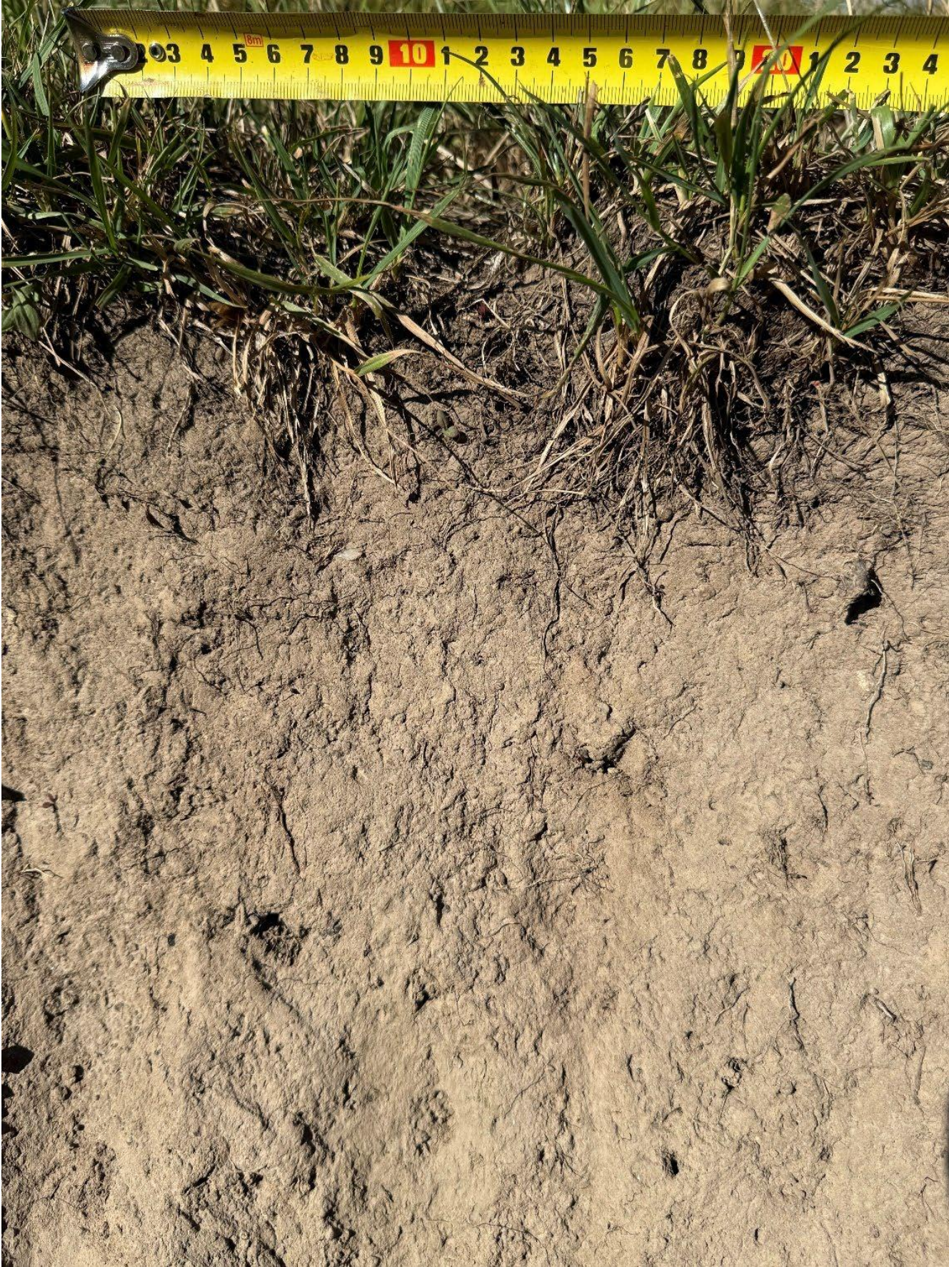
Image 8 Grey/brown clay loam dermosol soil present as per the Quamby soil profile present throughout the gently sloping and undulating ground extending along the central southern boundary area of the property. (taken on the site assessment 21/1/2025)
