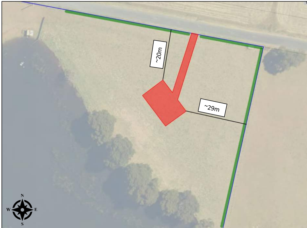
Figure 9. Setback distances of the proposed development area (red) from the title boundaries. Green lines indicate proposed pencil pine privacy screening (Source: LIST).
