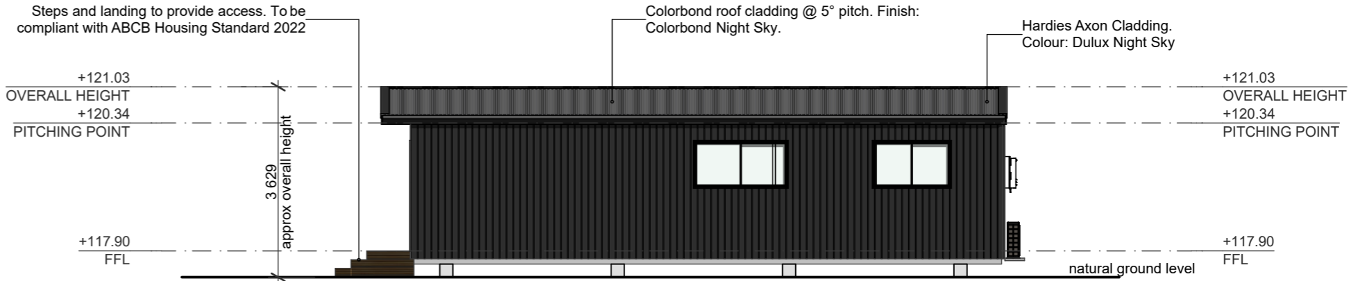
E-01 Western Elevation A02 Scale 1:100 @A3
