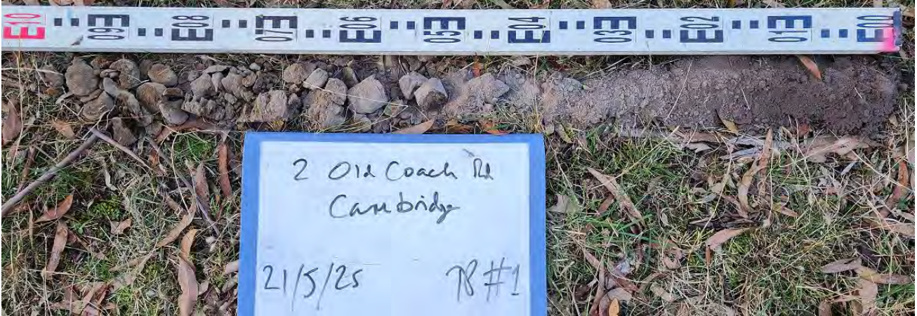
(above) Soil profile core sample from proposed land application area.
