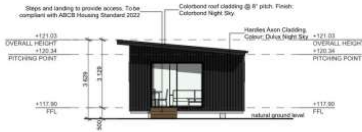
E-02 Northern Elevation A02 Scale 1:100 @A3
