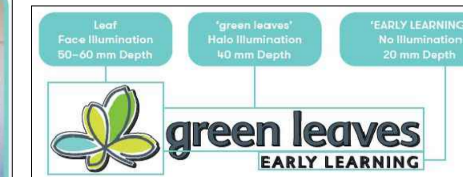
TYPICAL ILLUMINATED SET UP
