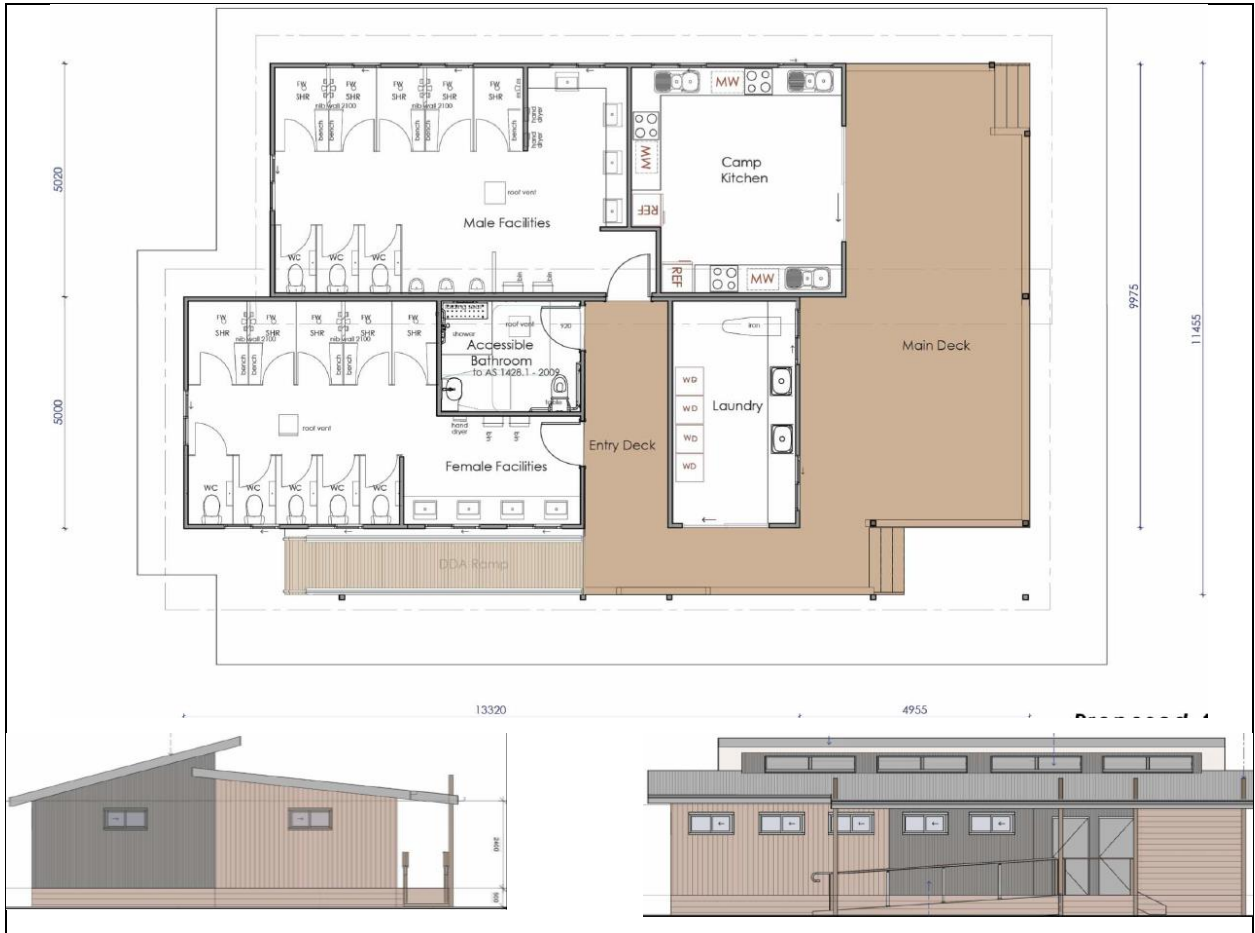
Figure 5 - Combined Amenities & Camp Kitchen - Floor Plan & Elevations - Sheets 8 & 9. Source: Green Hill Design
