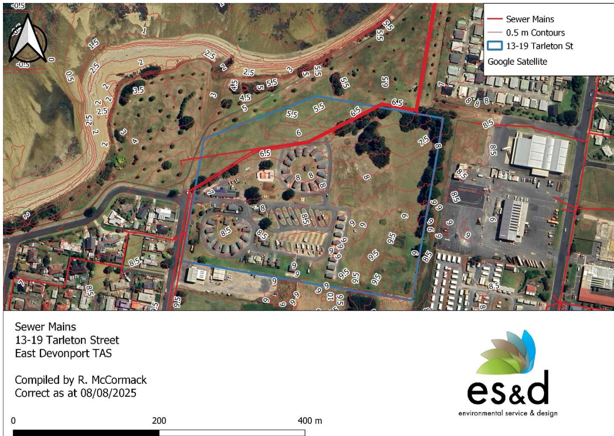
Figure 5: Sewer mains running through the site.
