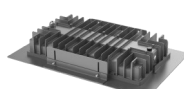
Recess Frame (Deep) Bracket-clamp retention for ceilings max. 40mm thick, fascia 580 mm x 370 mm, cut-out min. 510 mm x 320 mm
