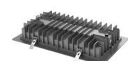
Recess Frame (Shallow) Spring-clip retention for ceilings max. 25 mm thick, fascia 535 mm x 325 mm, cut-out min. 510 mm x 300 mm
