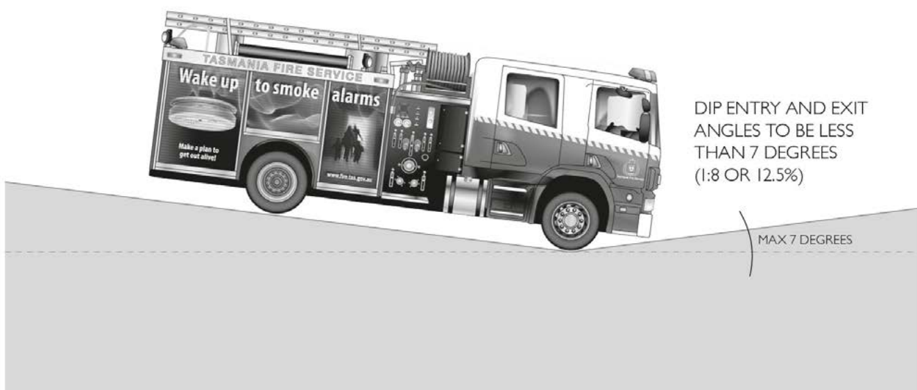
Figure 3 Dip approach and exit angles
