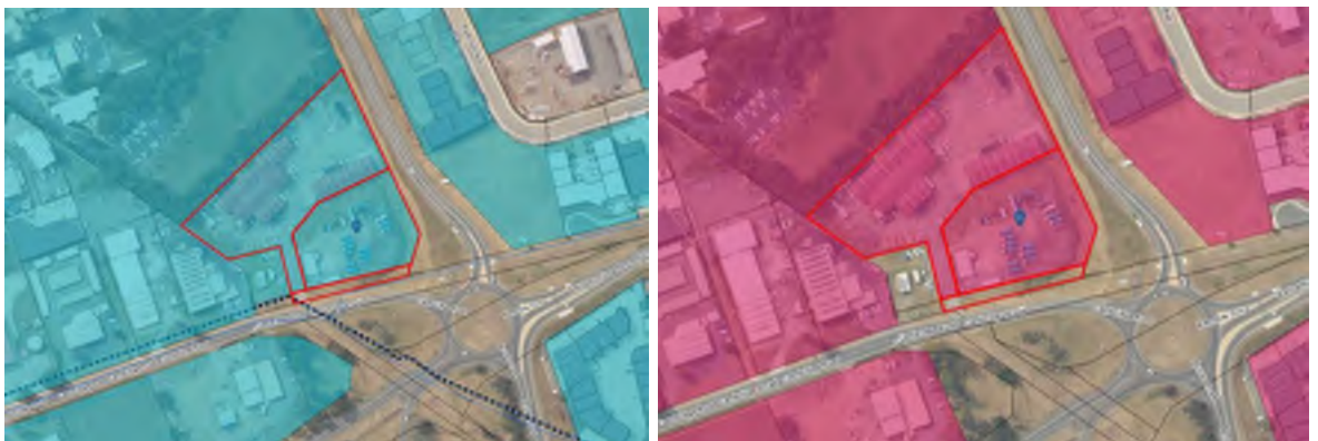
Figure 3: Water serviced land (blue) and sewer serviced land (pink) including mains (source: the Listmap, 2024)
