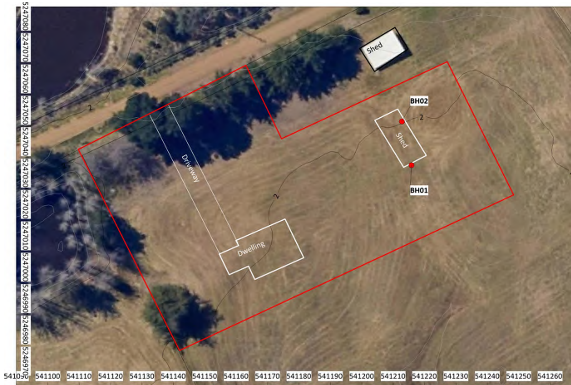
Figure 1 Site Borehole Locations
