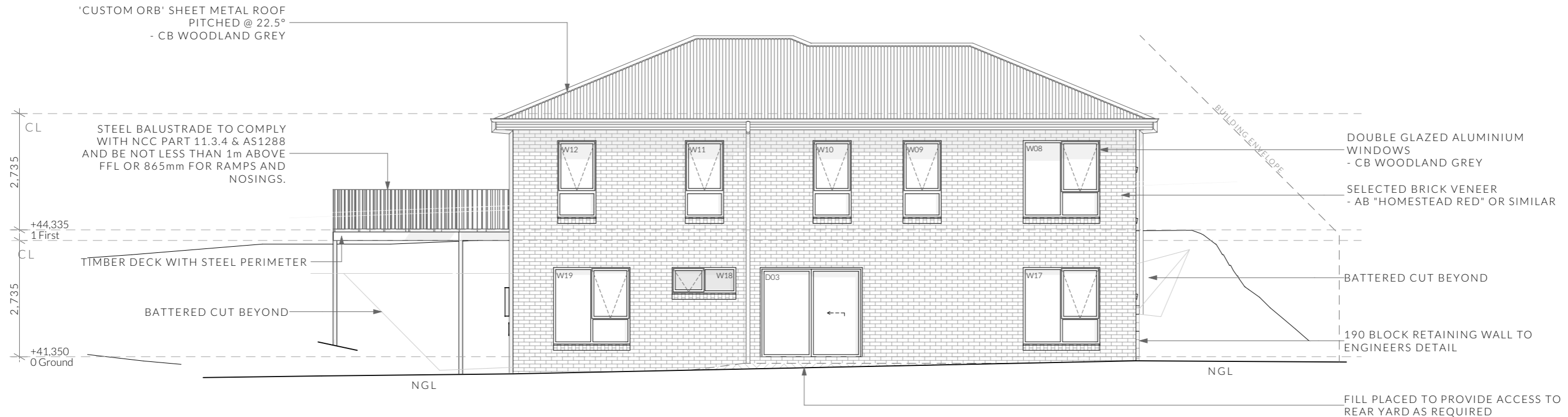
South West Elevation
