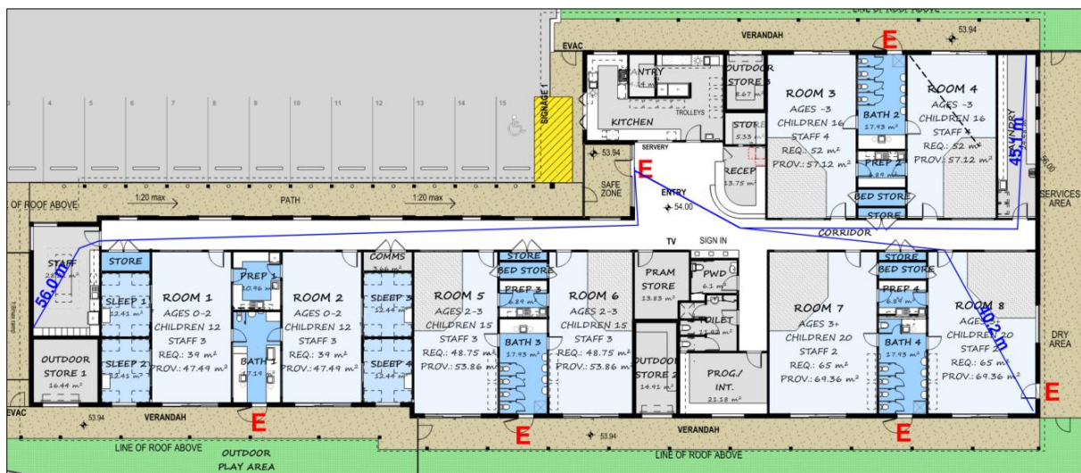
Figure 3: Hose lay measurement within the building (from the internal door of the air lock).
