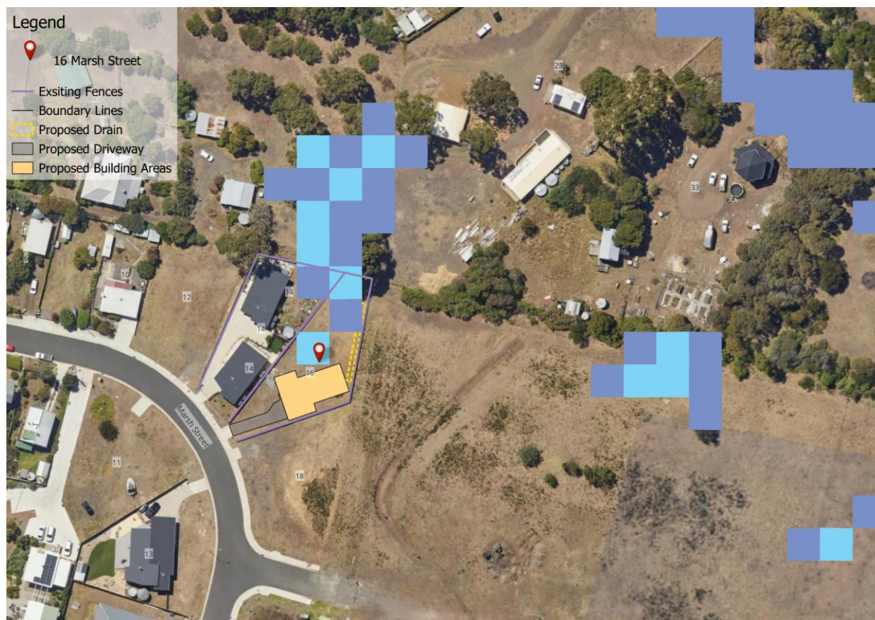
Figure 1. Proposed Development 16 Marsh Street, Opossum Bay showing 1% AEP Hazard rating (SES)
