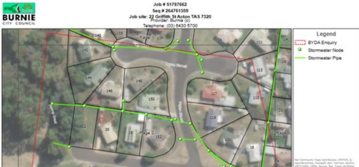
Figure 1: Stormwater asset plan retrieved from Burnie City Council via a BYDA enquiry (accessed: 25/11/2025).
