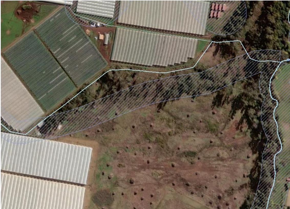
Figure 4 Proposed site location showing the waterway overlay not aligning to the hydrology data. Source LISTmap
