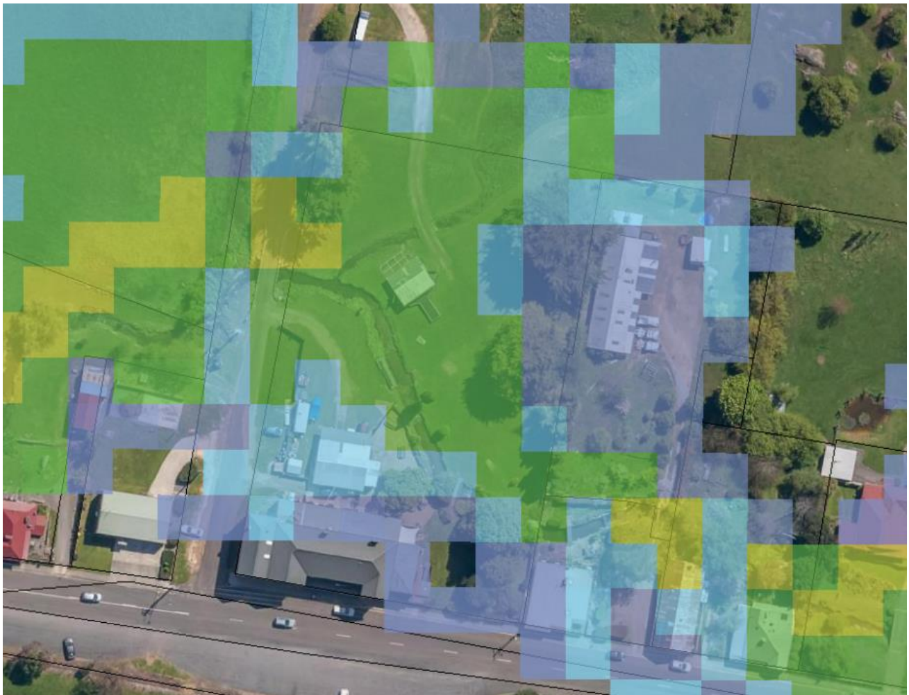
Figure 2. TSFM 1% AEP CC flood extent and hazards
