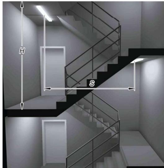
FIGURE 4.2 EXAMPLE OF EMERGENCY LUMINAIRES LOCATED ON INTERMEDIATE LANDINGS IN AN ENCLOSED STAIRWELL
