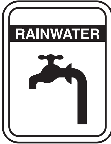
Figure 15.3.2.2 — Typical sign for rainwater outlets
