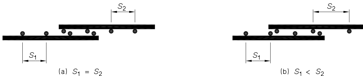
FIGURE 13.2.3 LAPPED SPLICES FOR MESH
