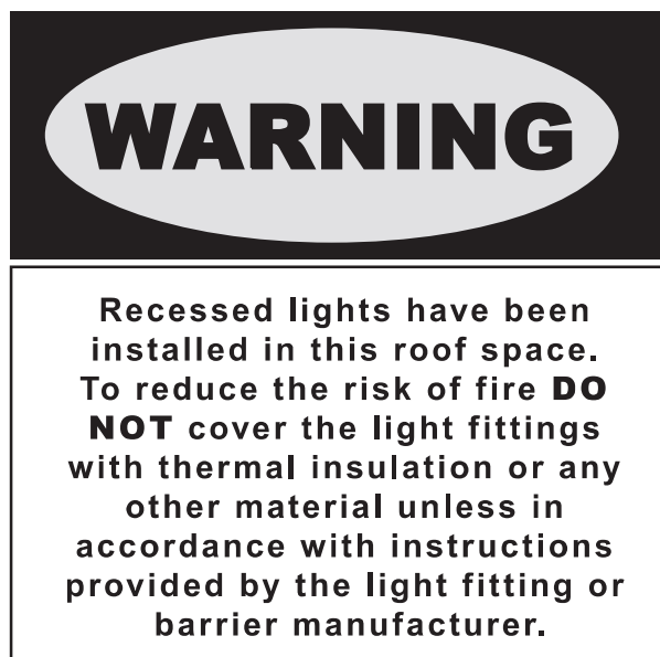
FIGURE A2 WARNING SIGN TO BE INSTALLED IN ACCESSIBLE ROOF SPACES CONTAINING RECESSED LUMINAIRES
