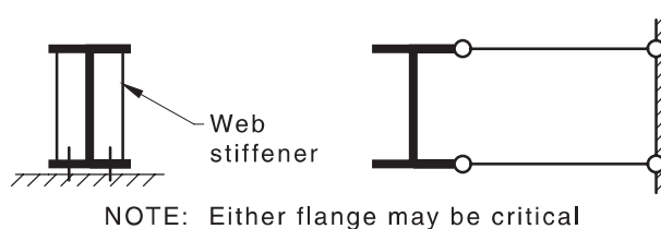
(a) Critical flange restraint, effective twist restraint
