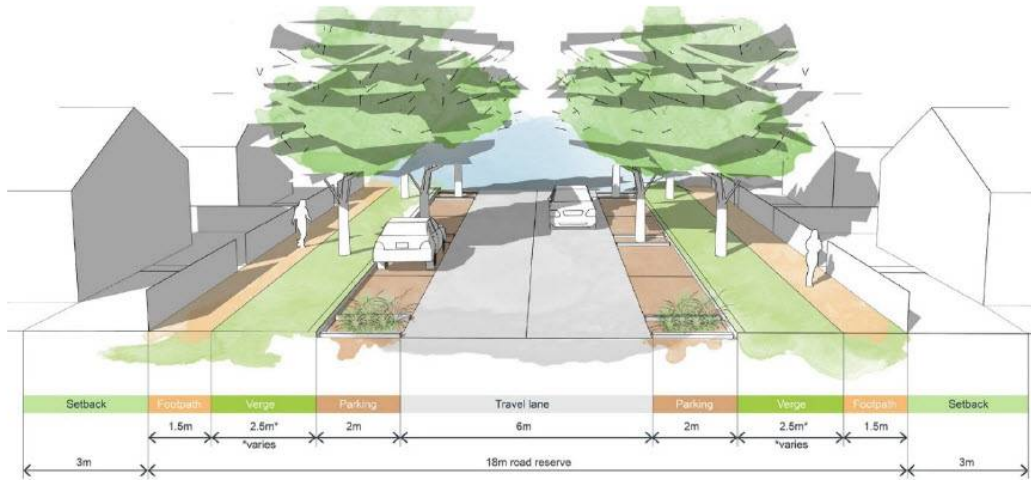
Figure DEV-S4.9 - Street typology for 18m wide reservation as required by clause DEV-S4.4.1, clause DEV-S4.7.3 P1(a), clause DEV-S4.8.1 P1(b), clause DEV-S4.9.3 A1.1(b) and P1(l), and clause DEV-S4.10.2 A1(b)
