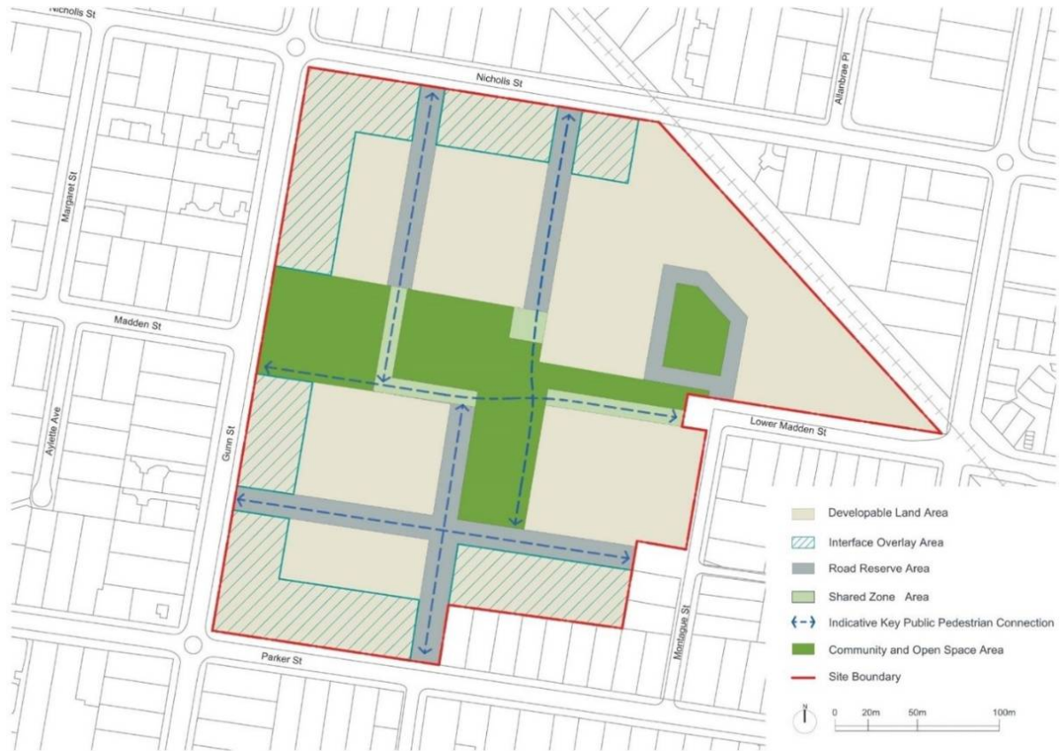
Figure DEV-S4.1 - Devonport Showground Redevelopment Master Plan Development Framework as referred to in clause DEV-S4.4.1, clause DEV-S4.6, clause DEV-S4.7, and clause DEV-S4.10
