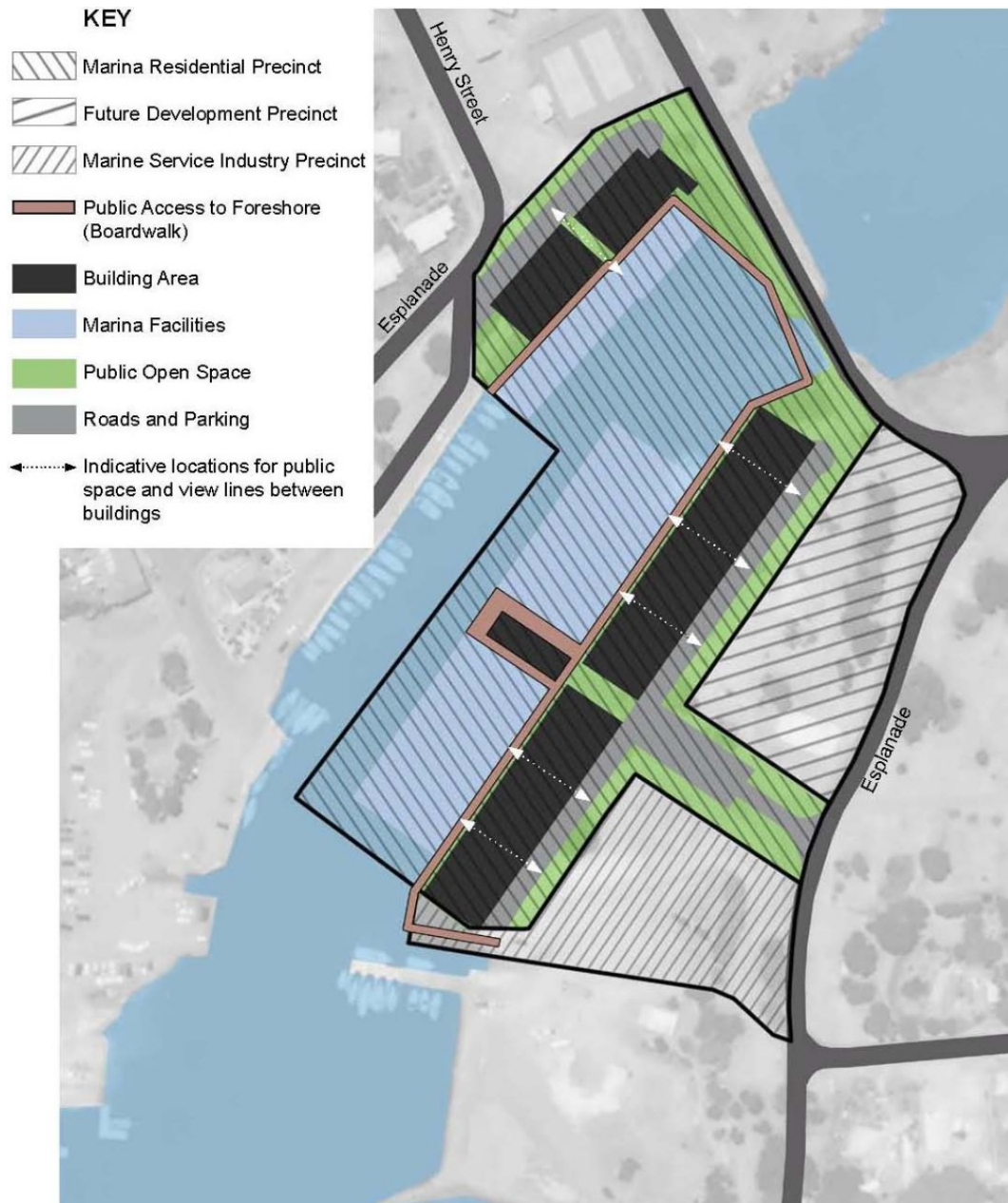
Figure GSB-S1.1 - Spring Bay Marina Precinct Plan as required by clause GSB-S1.2.1, clause GSB-S1.3, and clause GSB-S1.7.3 A2(a)
