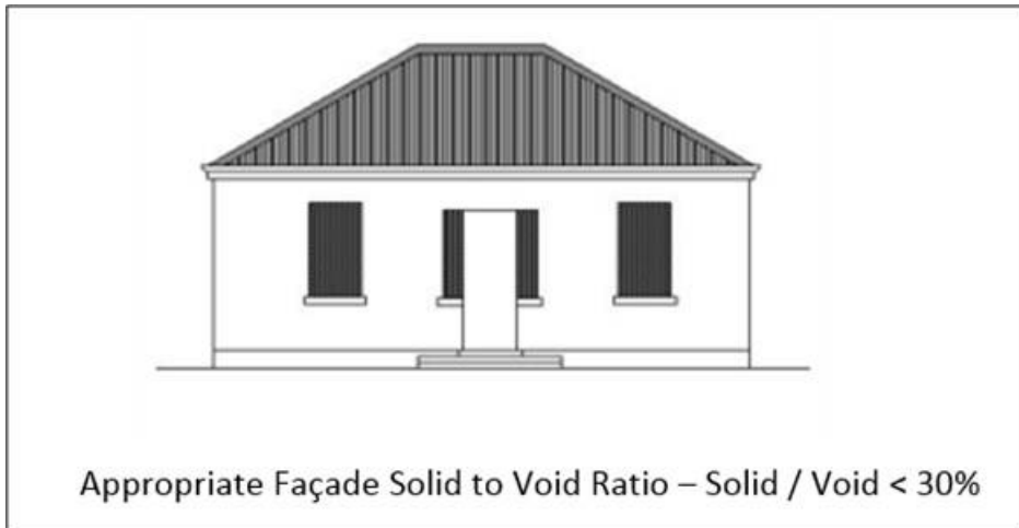
Figure NOR-S5.7.4(b) - Window shapes and styles as required by clause NOR-S5.7.4 A2
